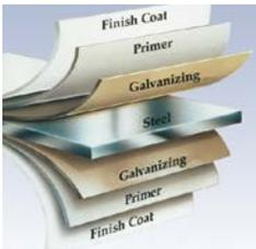
Steel skins are protected through a tough, layered coating system, including a hot-dipped galvanized layer, a protective metal oxide pretreatment and a baked-on primer and top coat.
